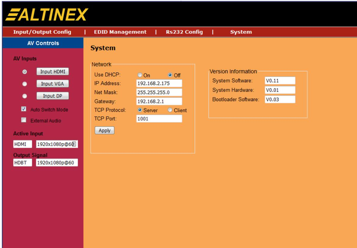
**System:** The System page configures the UT260-103 network settings and provides system details.
