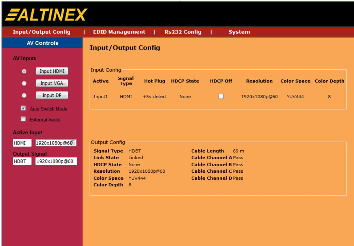
**Input/Output Config:** The Input/Output Config page provides the status of the TX/RX system.
