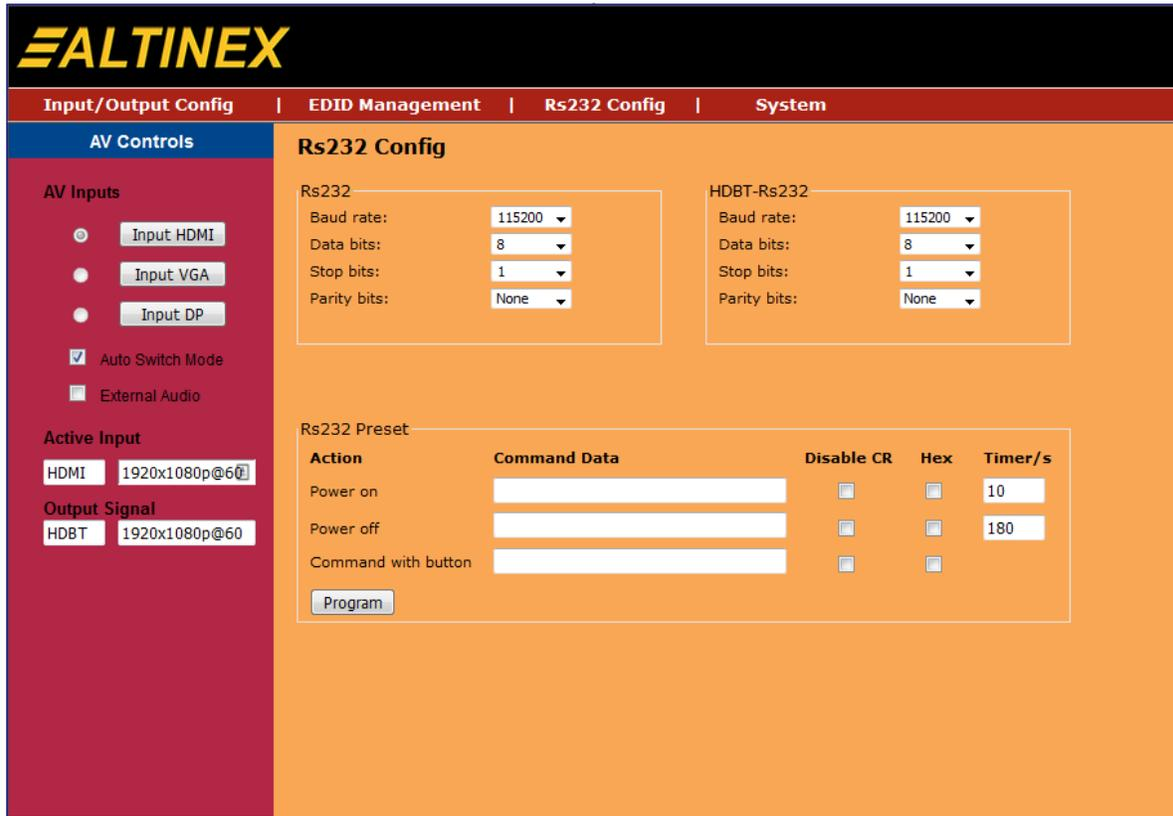
**Rs232 Config:** The Rs232 Config page may be used to configure the RS232 ports on the transmitter and receiver.
