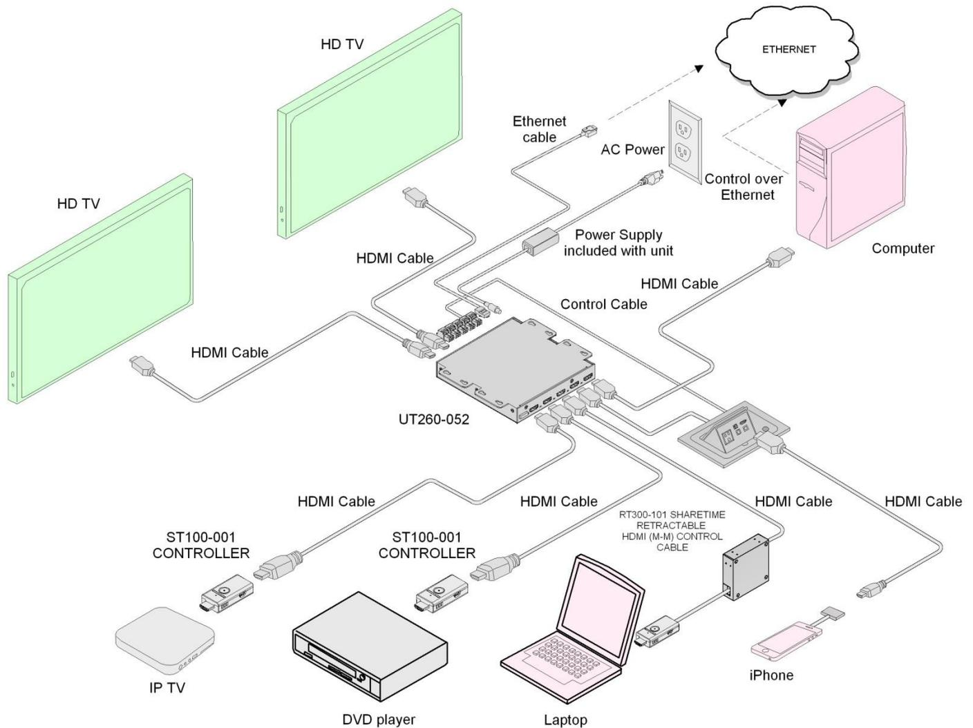
Having de-select enabled will allow the CEC controller to collaborate with the newly released UT260-052 5x2 HDMI switcher
